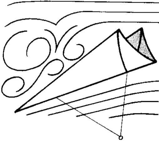
If the flyline and bridle hold the kite in the wind at an appropriate angle, then wind pressure is exerted against the sail. Lift results from this pressure being deflected across the face of the kite.
