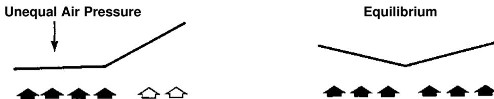
In other words, the greater surface area exposed receives greater wind pressure and tends to get pushed back into balance at the position of least resistance.
