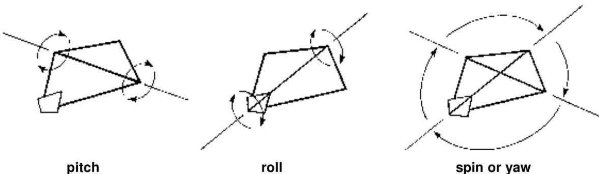
You're probably real confused now about boats, kites, pitches and yaws. The point is that unstable kites can move in a number of different uncontrolled directions. We need to look for design features which provide stability and control. Three that are particularly important are dihedral, balance, and the kite's angle of attack.
