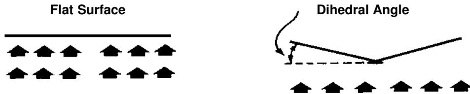
A flat surface naturally gives way to any pressure from the wind. Two flat surfaces, joined by an angle, move into a position that creates the least resistance. It works like a weather vane.
