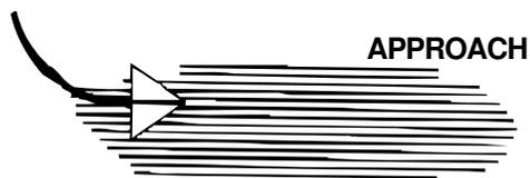
What you want the kite to do is pivot its nose vertical and stop in a stall at an altitude of not over 4 feet. Then immediately, PUSH or step forward. The kite will fly backwards down to a landing. Ta-daa!
